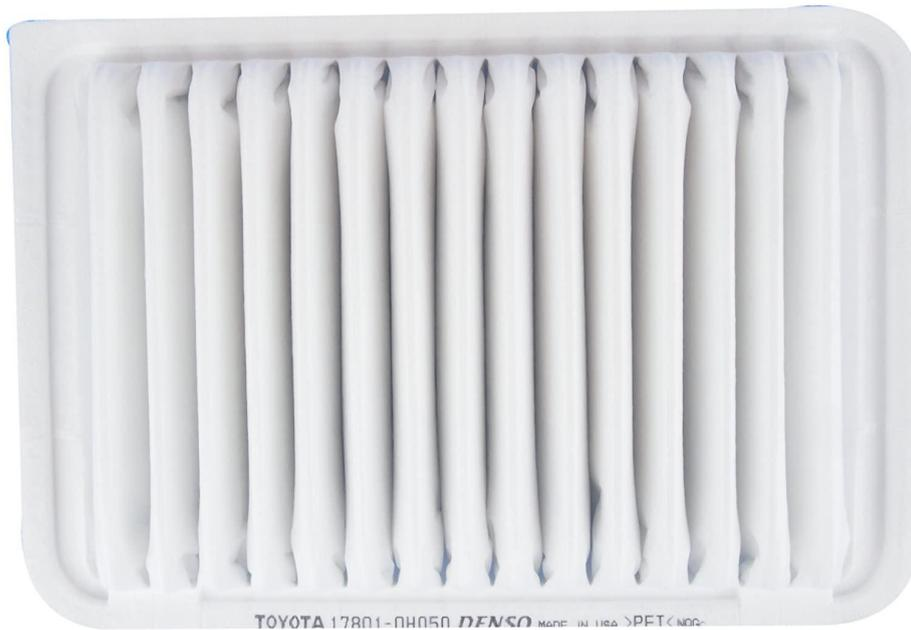
Toyota's engine air filter is specially designed for removing 99% of pollutants in the air before entering the engine.
